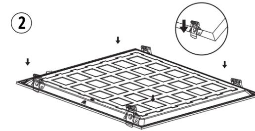
60x60  $\varnothing$  575x575mm      30x120  $\varnothing$  275x1175mm
