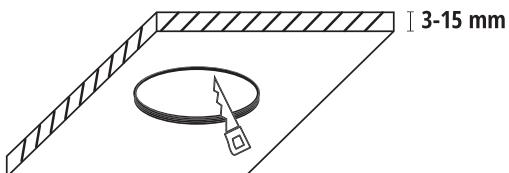
6W: Ø100-110mm, 12W: Ø140-160mm, 18W/24W: Ø195-210mm
